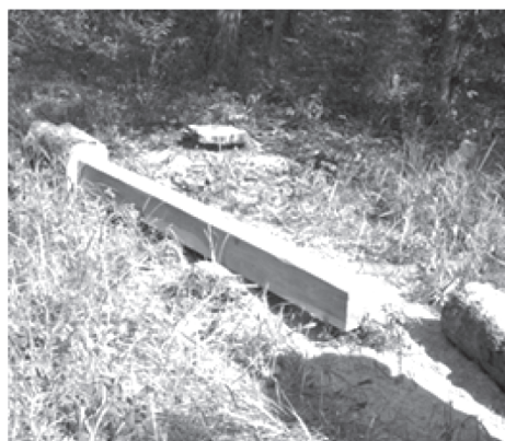
Figure 1 The timber size required for sawing standard 20 cm width wood out (left), and in situ processing of a pillar (right). The tree being processing is Erythrophleum succirubrus .
